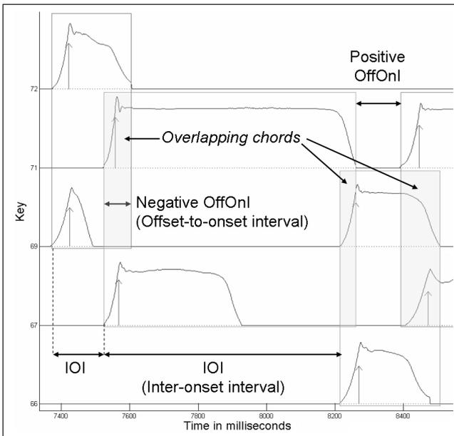
**Figure 5.** Pianoroll display of successive (framed) chords with their interval and overlap relations pointed out.
