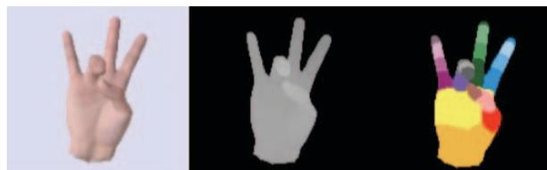
**Figure 13.** Depth field image retrieved from theKinect sensor and the semantic mapping of the for the hand shape by SigmaNIL.
