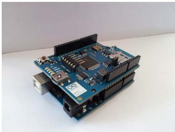
Figure 4. Arduino Uno with a Wifi Shield.
